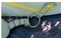
Metal clips to link booms.
