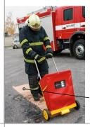
The cart design allows transfer from one place to another with no loss of the sorbent. Application of the material is highly effective because spreading is only enabled when the cart is being pushed forward, backing automatically prevents the drop of the material.
