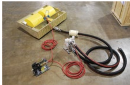
Pneumatically operated skimmer with diaphragm pump, air supply hoses and suction / discharge hose
