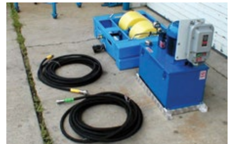
Electric hydraulic power pack, skimmer head and hydraulic hoses
