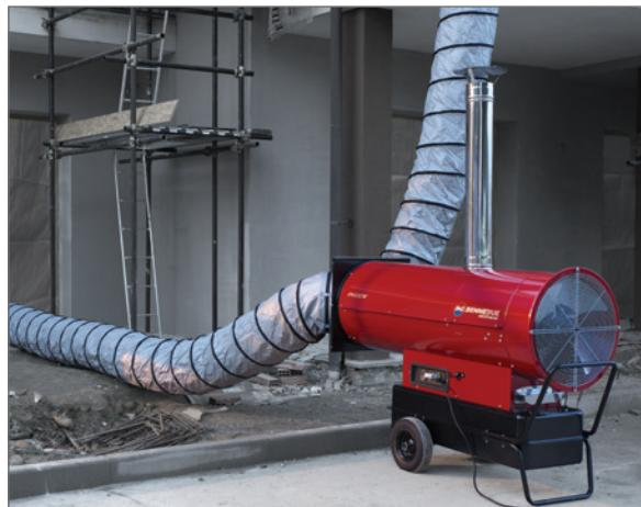
**PHOEN - INDIRECT COMBUSTION PORTABLE HEATERS
